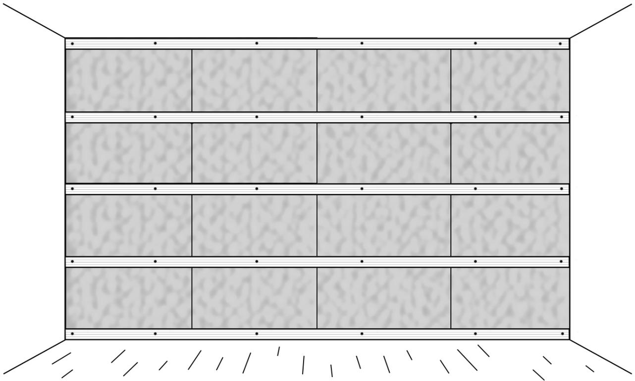
Insert a 45 mm. mineral wool between the battens. The mineral wool can be cut using a knife. The mineral wool is then squeezed in between the battens.
