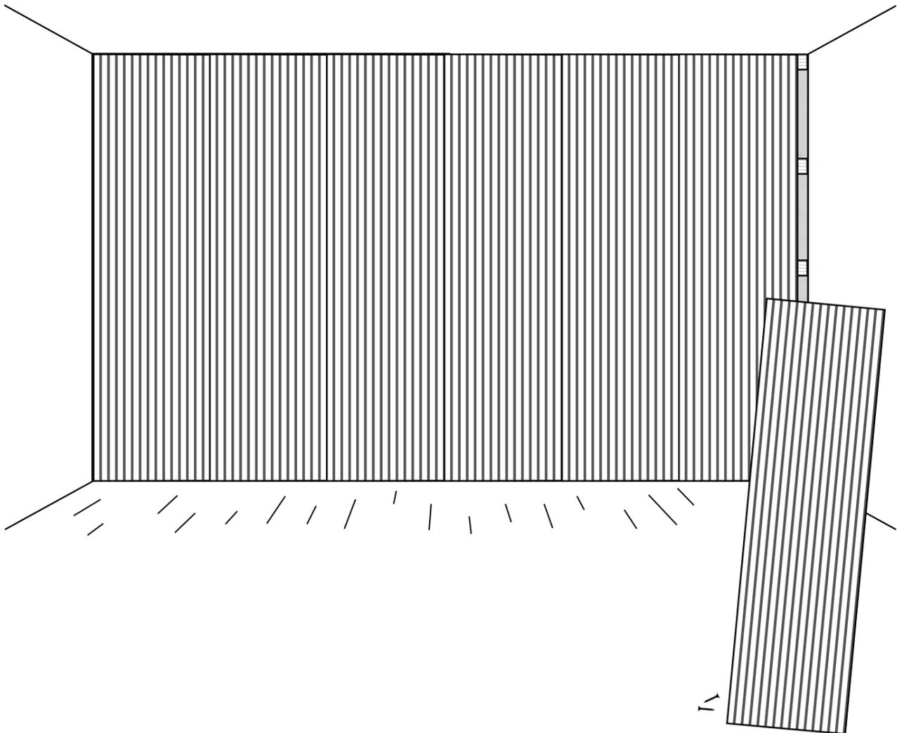
When reaching the end of the wall you might need to adjust the panels in order to make the panels fit.
