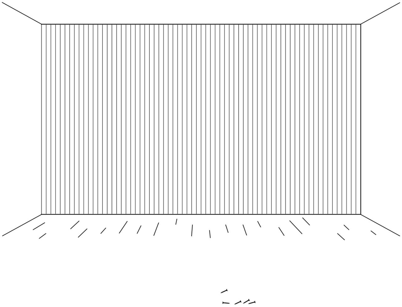
Mount the Akupanel on the wall by drilling the black screws (35 mm.) through the black felt and into the battens. We recommend 15 screws per Akupanel.
