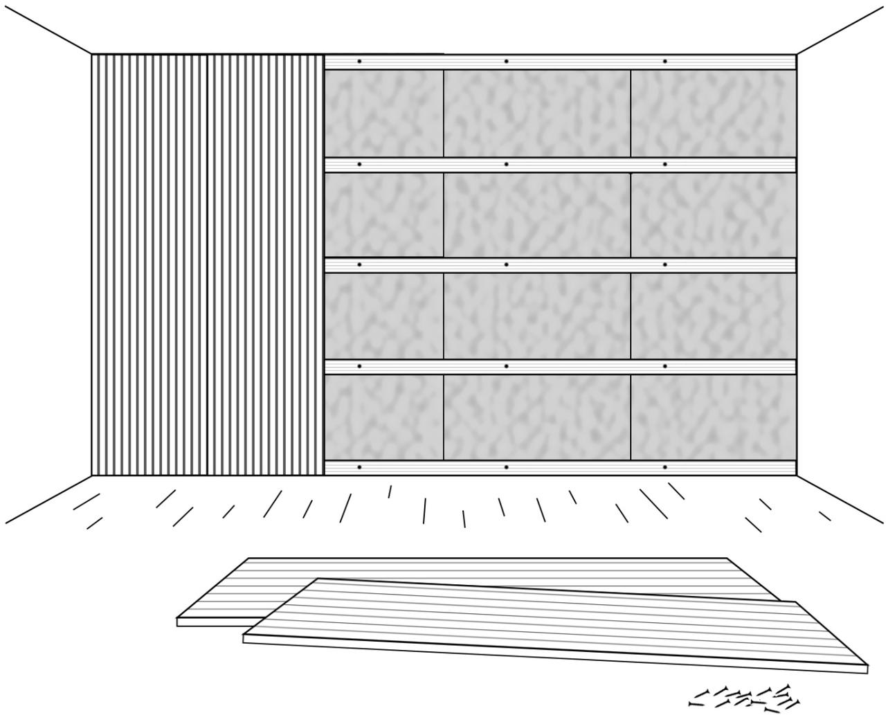
The panels have a felt side and a lamella side. When you mount the panels in continuation of each other you need to make sure that the felt side from one panel is flush with the lamella side on another panel so that there is about 12 mm between the lamellas in the jointing.
