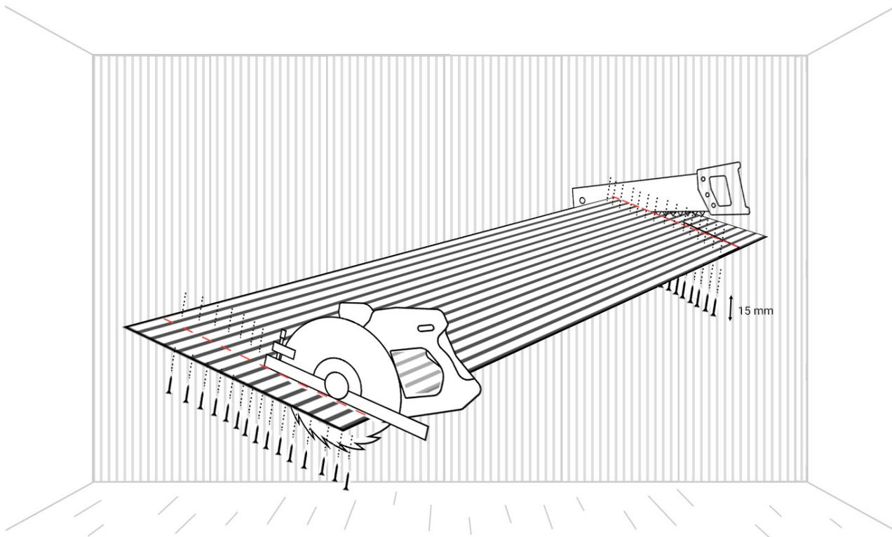
If you need to adjust the height of the Akupanel you can do so by using a saw like for instance a circular saw or a foxtail. Mark the cutting line on the panel with a pencil.
