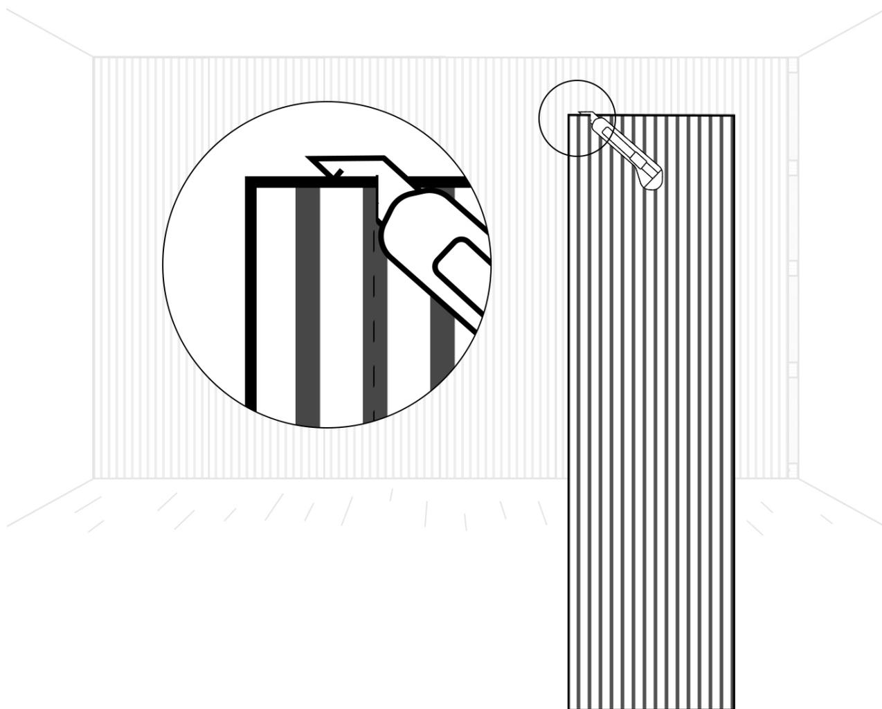
Adjusting the akupanel sideways is done by cutting the panel in the felt using a knife.
