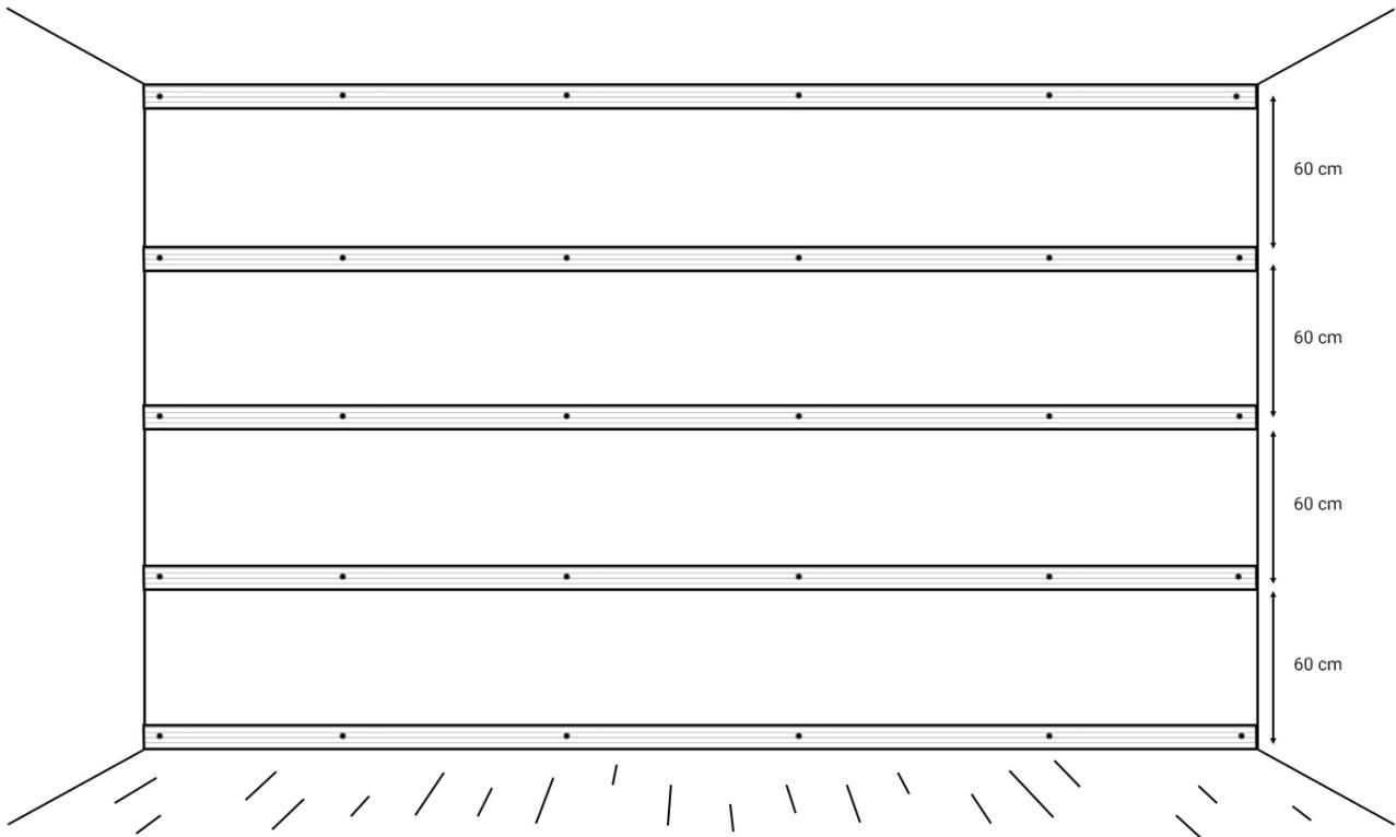
The first thing you need to do is to mount battens on the wall. This enables you to drill the screws through the felt of the akupanel and into the battens. Depending on the wall you will need plugs and screws that fits accordingly to your wall type. We recommend that you keep a distance of 60 cm. between the battens.
